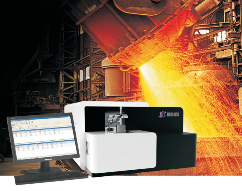
**W5** Optical Emission Spectrometers (Arc/Spark-OES)
